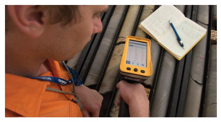
Vanta<sup>™</sup> analyzers offer rapid return on investment (ROI) by providing users with "decision quality" geochemical data much faster than traditional laboratory techniques. Rapid, accurate decision-making at the exploration stage enables field time to be used more effectively, maximizes exploration (drilling and analytical) budgets, and advances project timeframes.
