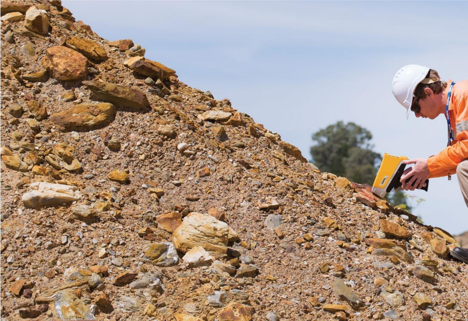
The Olympus Vanta™ handheld XRF provides immediate, on-site elemental measurements for a range of geochemical applications. Vanta analyzers provide power and flexibility across the entire mineral resource cycle:
