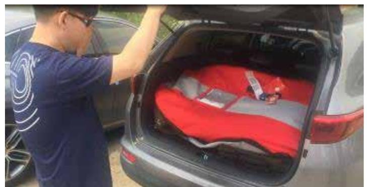
The board is able to fit in the boot of any standard sized car and weighs 8Kg. The board carry bag includes integrated shoulder straps. The controller, thrusters and power supply fit in a waterproof case with integrated wheels, dimensions D280mm by H560mm by W400mm, weight 16Kg.
