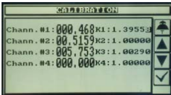
CALIBRATION MENU: The software allows to check and calibrate the 4 available channels.
