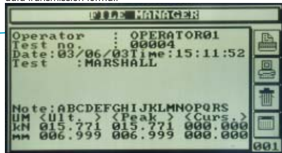
FILE MANAGER: It is possible to save the test or to recall a test previously saved. The tests can be printed or downloaded to a PC.
