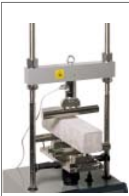
6) 70-T0108/E equipped for flexural tests on concrete beams (centre point loading only)
