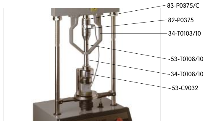
13) 70-T0108/E equipped for compression test on mortar
