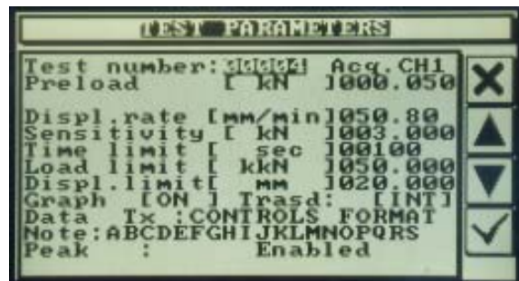
TEST PARAMETERS: It is possible to introduce peak sensitivity and preload, to enable peak and graph during the test, to choose data transmission format.
