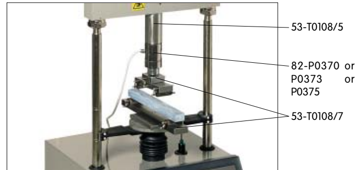
11) 70-T0108/E equipped for testing the flexural strength of soil cement specimens
